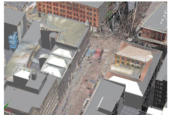
Overlay of 3D model and point cloud scan data
